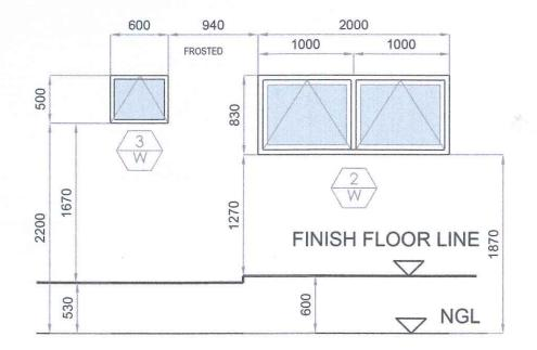
W3 ELEVATION **W2** ELEVATION TYPE: UPVC GREY AWNING WINDOW 10mm THK CLEAR GLASS TYPE: UPVC GREY AWNING WINDOW 10mm THK CLEAR GLASS QUANTITY: 1 SET QUANTITY: 1 SET LOCATION: GUARD HOUSE LOCATION: GUARD HOUSE
